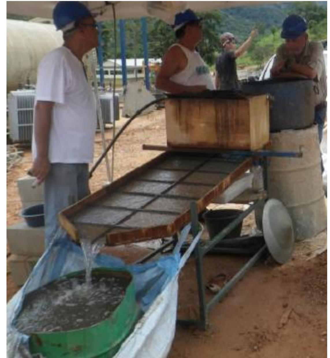
Piloting new technologies to reduce the use of mercury in small-scale mining in Brazil
